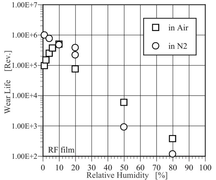
Fig.3 Wear life against relative humidity of RF film
