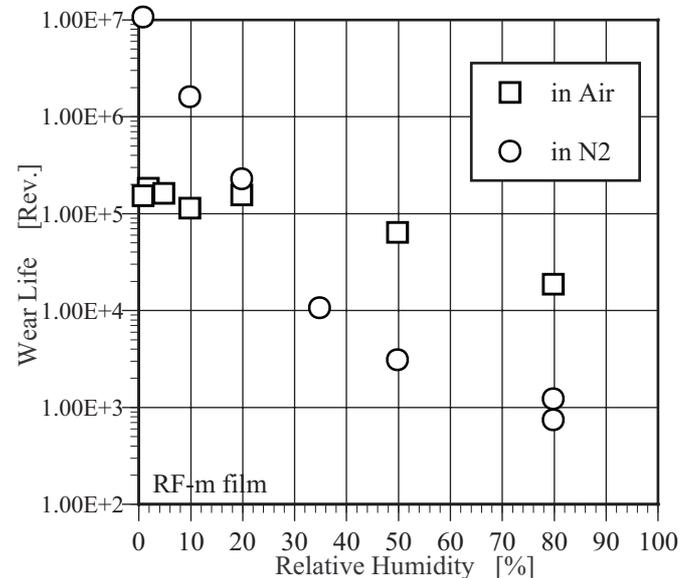
Fig.4 Wear life against relative humidity of RF-m film
