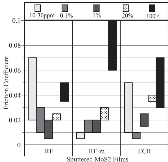
Fig.2 Friction coefficient of films in various oxygen concentration
