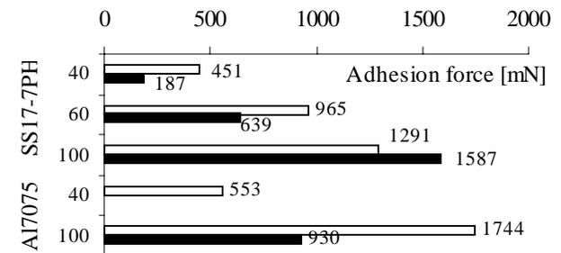
Fig.4 Adhesion force as function of static load (in %EL) and impact energy ( $49 W_Y$  ,  $200 W_Y$  <). Comparison of SS17-7PH and Al AA7075 (Al7075). In terms of bond strength, Al sticks to itself twice as strong as SS17-7PH.
