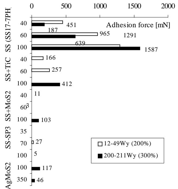
Fig.3 Adhesion force as function of static load (in %EL) and impact energy (SS = SS17-7PH). Coatings on discs (TiC and MoS<sub>2</sub>) reduce adhesion. MoS<sub>2</sub> acts in both types: as coating and in composites.
