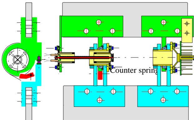
Figure 6 : one-shot hinge adapted to reversible motion.
