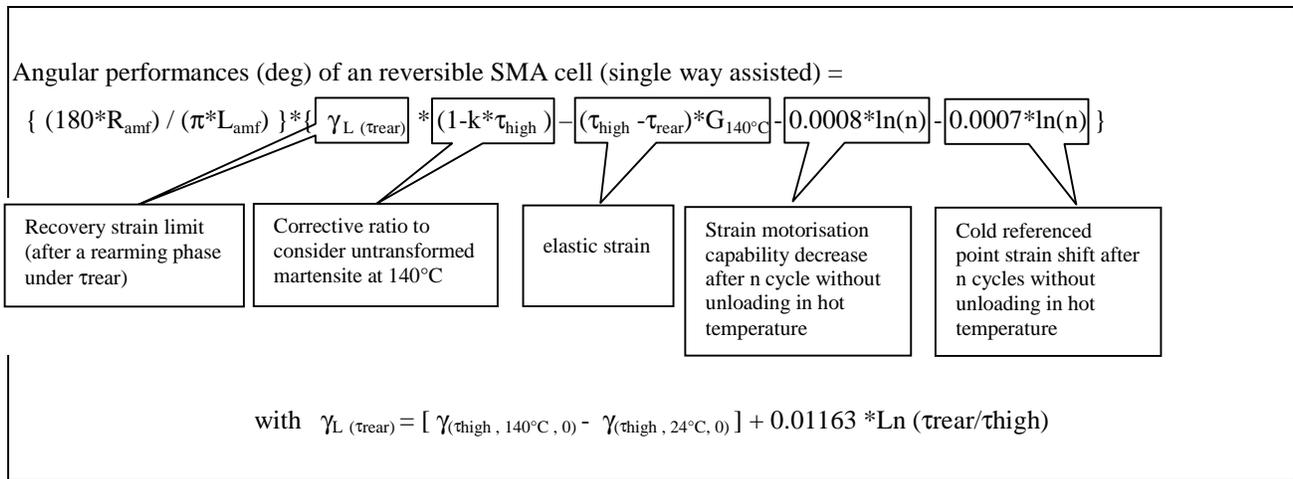
Figure 5 : synthesis of the reversible SMA cell model.
