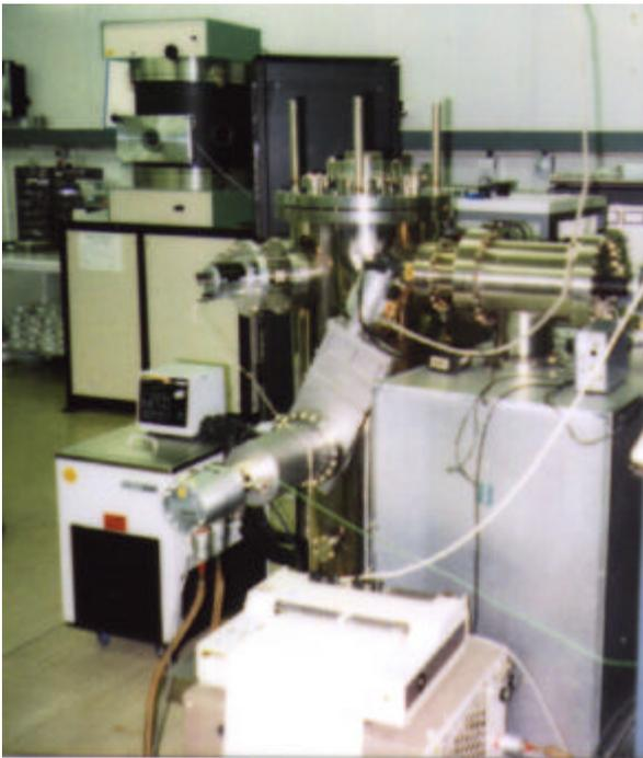
Figure 6. Thermal-Vacuum chamber at ESTL.
