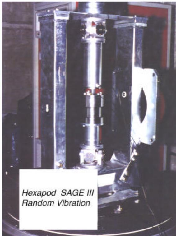
Figure 4. Random vibration test fixture.
