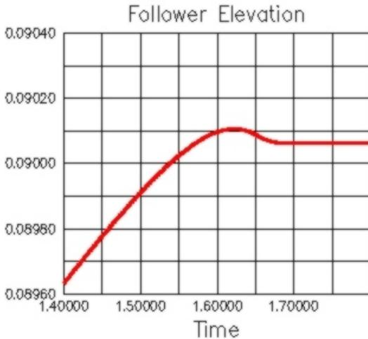
**Figure 10** The Follower elevation / cam detent
