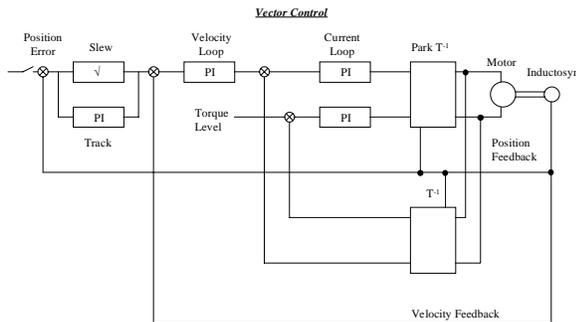
Figure 11. Block Diagram of DSM Control
