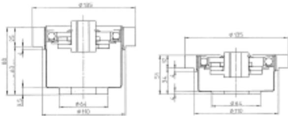
Figure 5. Short flexspline design
