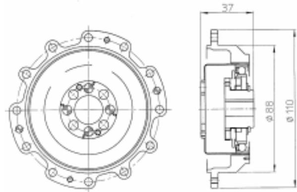
Figure 7. Component set with modified circular spline
