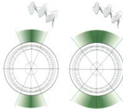
Figure 4. Comparison of involute and IH tooth profiles
