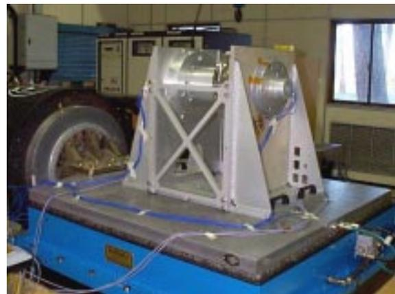
Figure 15: BBM instrumented for vibrations
