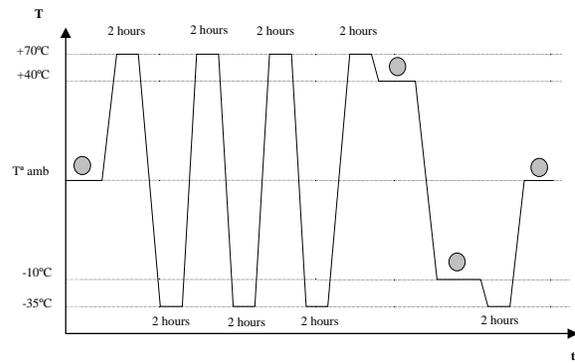
Figure 17: Thermal cycling test profile
