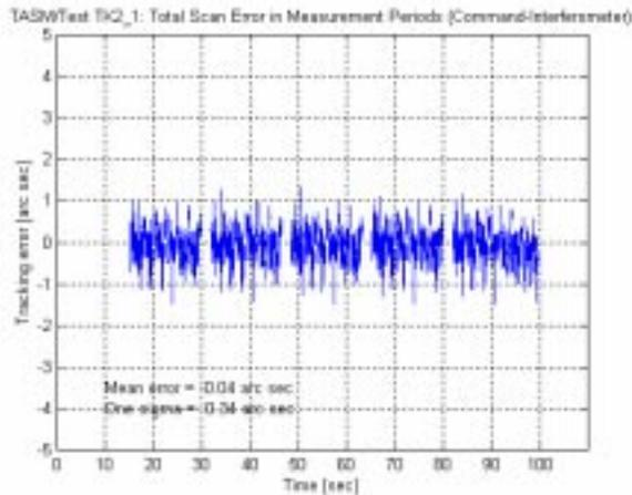
Figure 14: Absolute scan error in discrete mode
