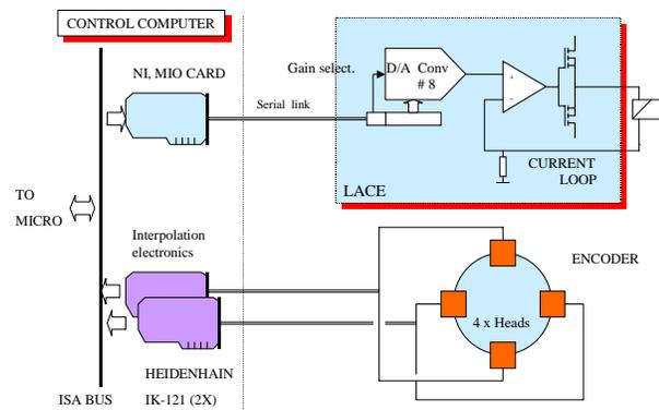
Figure 8: Electronics configuration
