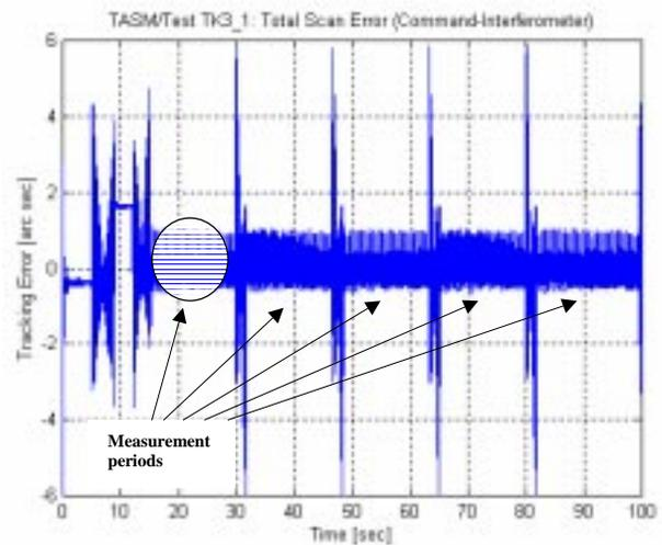
Figure 12: Absolute scan error in continuous mode
