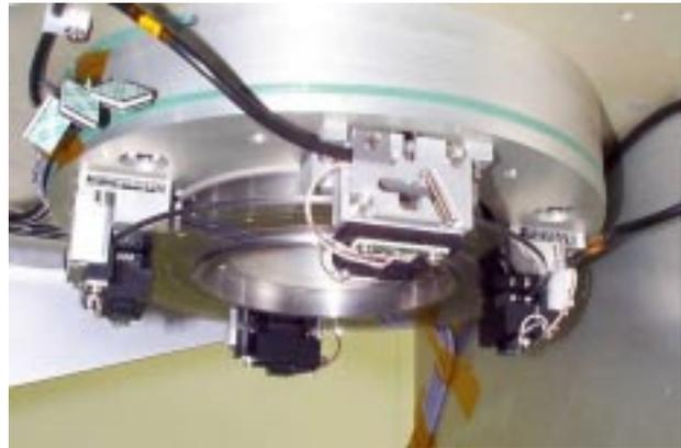
Figure 4: Flexural hinge-encoder assembly
