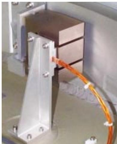
Figure 6: E-shaped voice coil actuator
