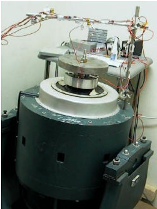
*Figure 5.: The LTV model A286 shaker*
