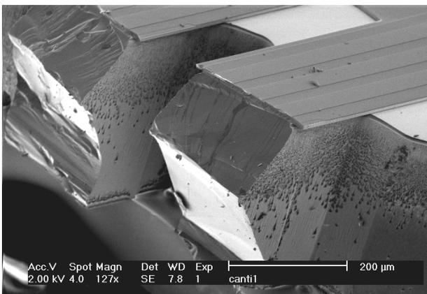
**Figure 4.** SEM image of the cleaving edges produced when breaking off the thick support beams for a cantilever exchange. The electrical paths for contacting the piezoresistors are visible on top of each beam..
