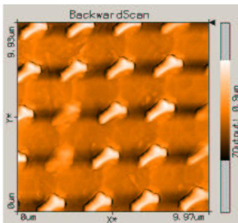
**Figure 11:** AFM image of a tip calibration sample taken with a quartz contaminated tip. The fuzziness and reduced height of 2 repeated features on the image results from blunt tips of the calibration sample.
