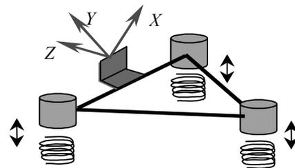
**Figure 5:** Schematic view of the scanning principle. 3 magnets are placed in a triangular configuration and attached to a spring-loaded platform. A coil is placed under each magnet. By supplying the right currents to the coils, one can describe a linear motion in x, y and z at the sensor array position.
