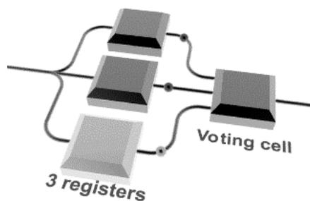
**Figure 6:** Illustration of the triple voting scheme. Even if one of the three register cells has a falsified bit induced by a heavy ion impact, the voting cell will still transfer the correct information..
