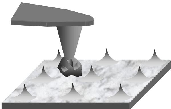
**Figure 7:** Schematic principle of the reverse imaging technique. The use of an array of sharp tips as a measuring sample will produce an AFM image with repeated topography of the particle sticking on the AFM tip since it has a bigger curvature than the calibration tips.
