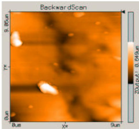
**Figure 10:** AFM image of quartz particles taken in tapping mode with a clean and sharp AFM tip.
