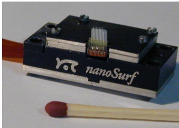
*Figure 2: Front view of the electro-magnetic scanner with mounted AFM chip. Wire-bonded connections link the silicon chip to the flex-print that comes out on the side of the scanner.*
