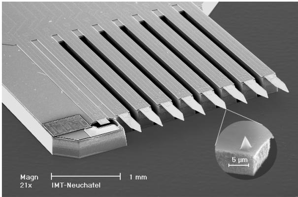
**Figure 3:** SEM image of the AFM chip. 8 cantilevers and tips are located at the edge of support beams. Integrated piezo-resistors for deflection sensing have been implanted onto each cantilever. A reference resistor implanted on an ultra-short cantilever and surrounded by a safety bar will compensate thermal drifts.
