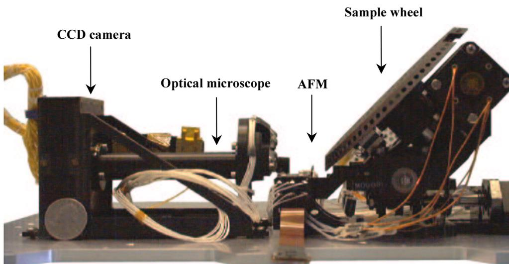
*Figure 1: Photograph of MECA's microscopy station with the cover removed.*
