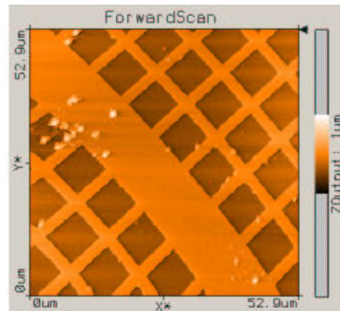
**Figure 8:** AFM image of a 10  $\mu\text{m}$  calibration grid with 200 nm step height.
