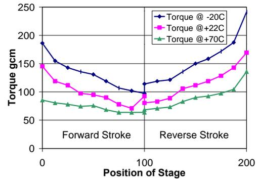
Figure 5 EQM Translation Stage Drive Torque v Position
