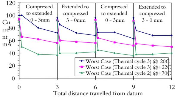
Figure 4 Summary of Current v Deployment Distance (EQM Unit)
