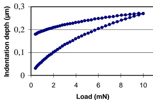
Fig. 4: Load-indentation depth curve for  $MoS_2$ -WC.
