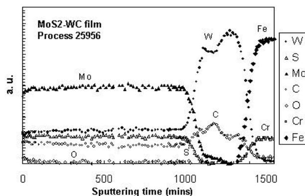
Figure 1: XPS element intensity depth profile of MoS<sub>2</sub> / WC film as a function of the sputtering time.
