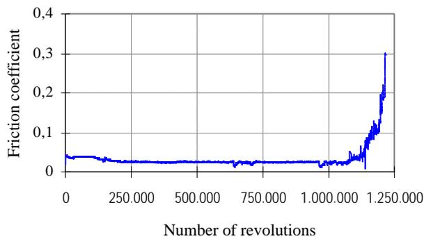
Fig. 5: Characteristic mean friction curve from MoS<sub>2</sub>-WC thin film when tested under vacuum conditions at 0.75 GPa.
