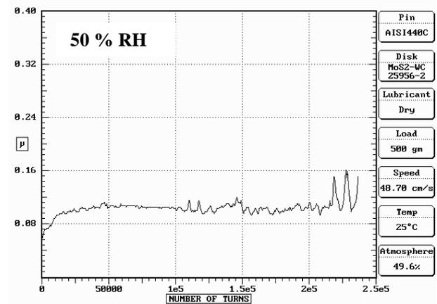
Fig. 6: Characteristic friction curve from MoS<sub>2</sub>-WC thin film when tested under atmospheric conditions, 50% RH.
