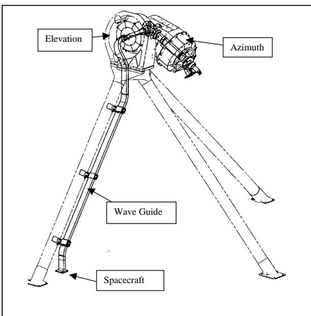
**Figure 22 – Waveguide**
