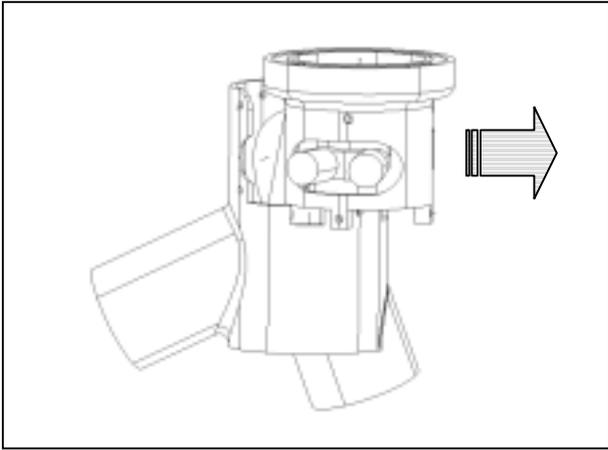
**Figure 14 - Removal of potting unit of tripod HRM**
