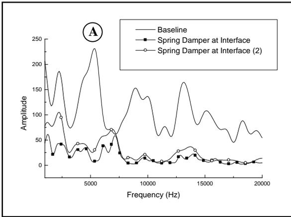
**Figure 9 – Fourier Transform of Shock Spectra**
