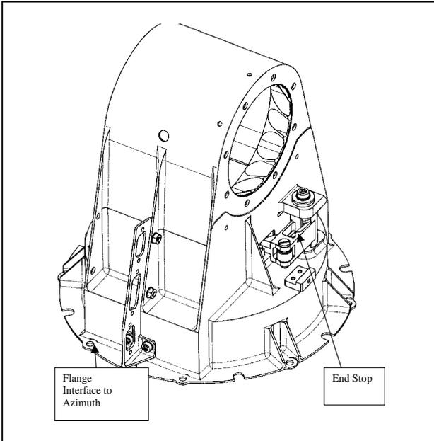
**Figure 17- Azimuth Bracket**
