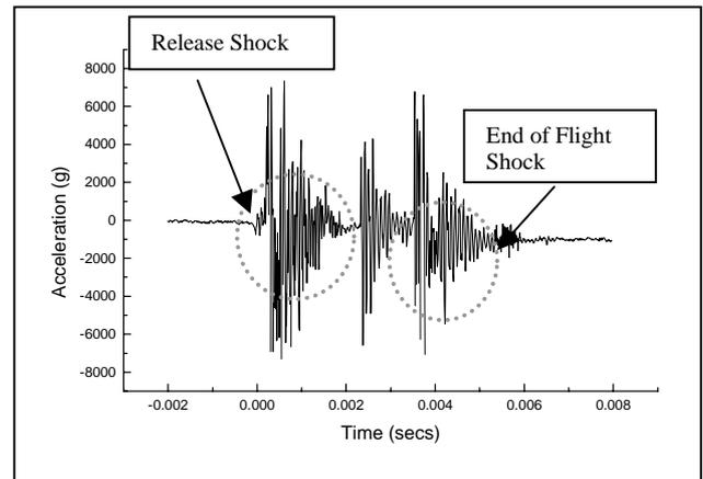
**Figure 4 – Shock Response without Damping**
