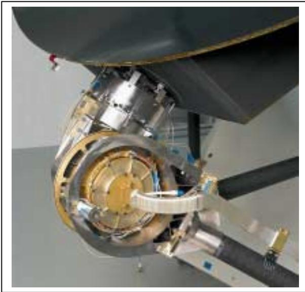
**Figure 21 – Antenna Pointing Mechanism**
