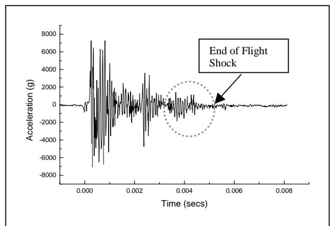
**Figure 5 – Shock Dampened by Usage of Honeycombs**
