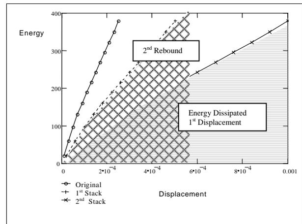
Figure 8 – Energy Absorption Curves of Damper
