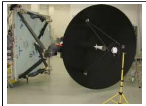
***Figure 25– Flight Model of The High Gain Antenna***
