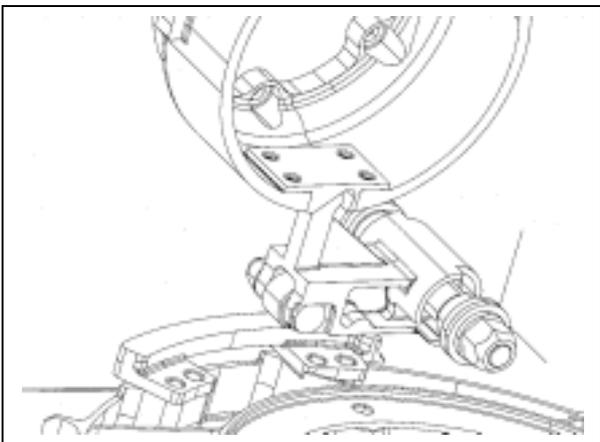
**Figure 18 – End Stop Mechanism**
