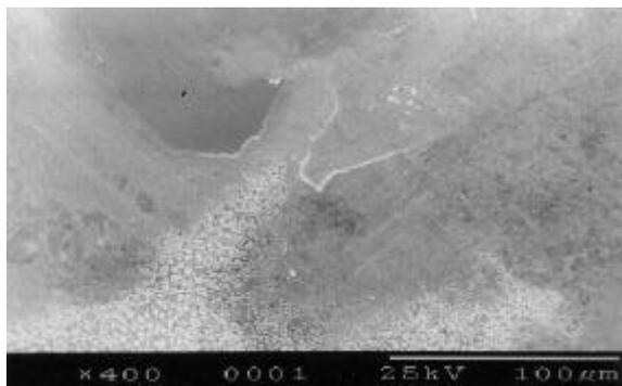
**Figure 8** Scanning Electron Micrograph of the Edge of elliptical Zone of Lead lubricated Raceway shown in Figure 7
