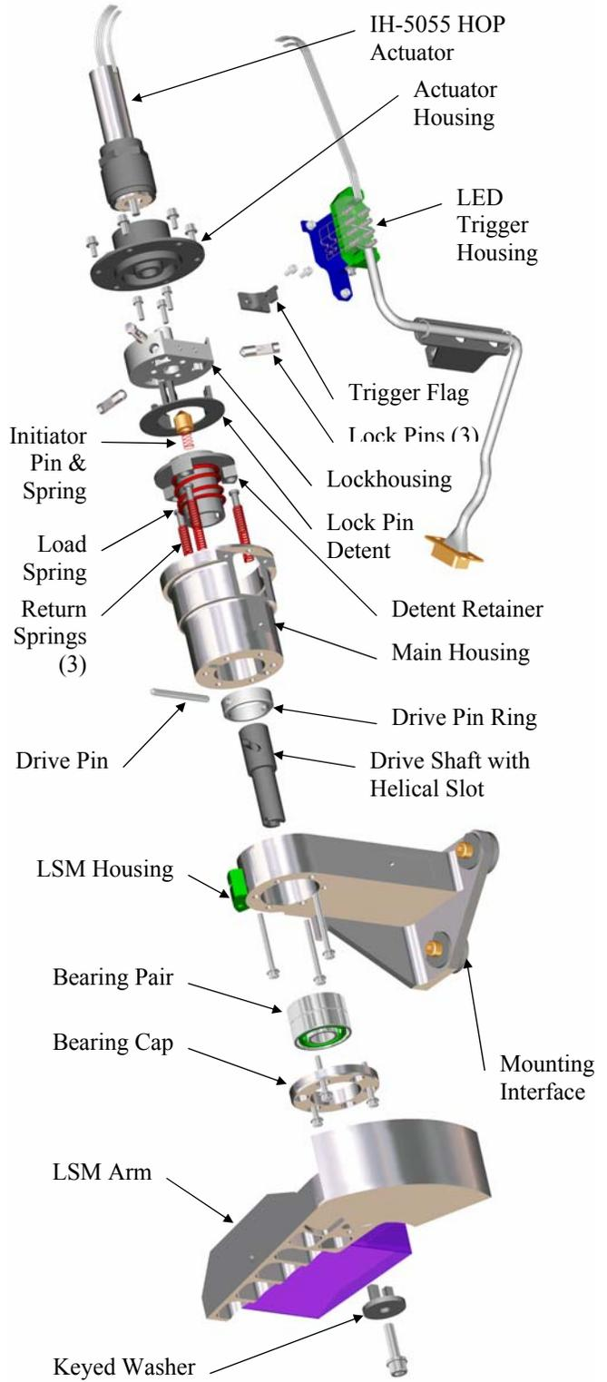
Figure 2. Exploded LSM
