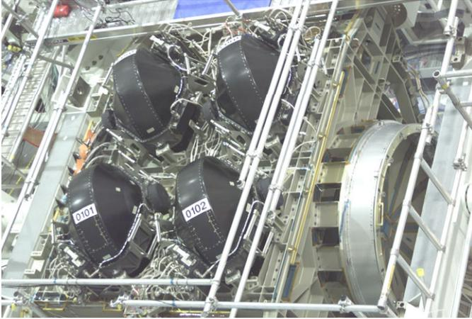
**Figure 1: CMGs 1-4 Mounted on Z1 Truss**
