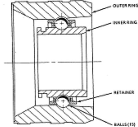
**Figure 2b: CMG Spin Bearing Assembly**
