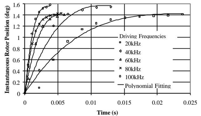
Fig.3 Dynamic behavior of the actuator for various driving frequencies in the range 20 to 100 kHz [6].
