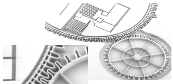
Fig.6 Self-actuated space mechanism including gear box reduction (components are 50 microns thick).
