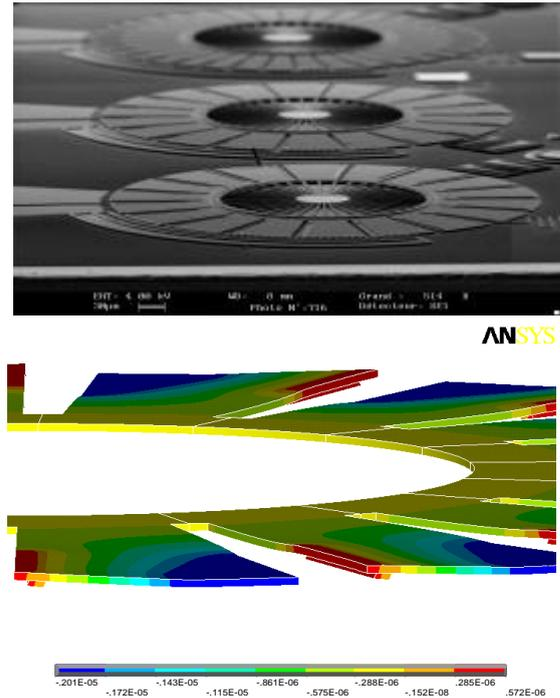
*Fig.1 Surface-micromachined electrostatic actuators using contact interactions on the wafer level*
