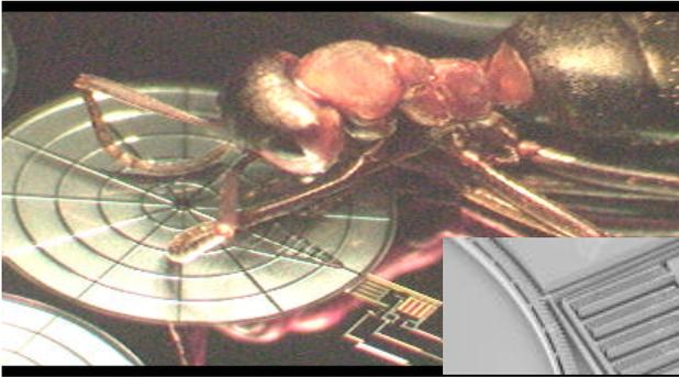
*Fig. 7 Ant playing with an high-aspect ratio MEMS-based mechanism realized on an SOI wafer. The wheel (2 millimeters/ 50 microns thick) integrates several hundreds teeth.*
