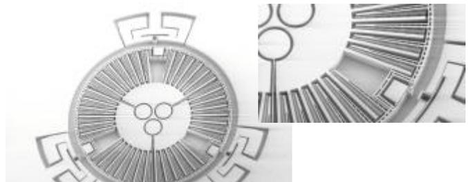
Fig.5 High-aspect ratio electric field driven SOI actuator for active control of read/write magnetic head.
