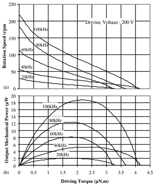
Fig.4 (a) Torque/ speed characteristics of electrostatic micromotors using stator/ rotor contact interactions, and (b) output mechanical power as a function of the driving frequency.
