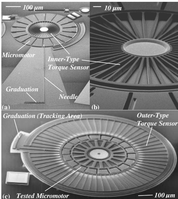
Fig.2 (a) and (b): Micrometer size test structure combining annular electrostatic micromotors with inner-type and outer-type elastic torque sensors, (c) magnified SEM micrograph showing an inner-type polysilicon torque sensor. After [5] and [6].
