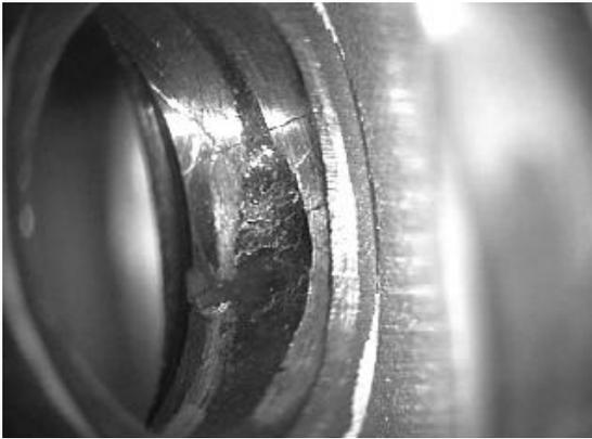
Figure 9 LTM3 lower cage pocket showing wear marks
