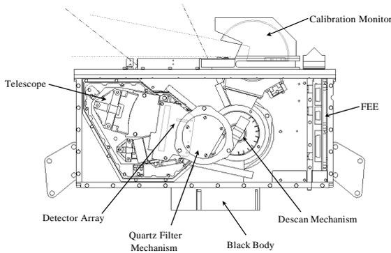
Figure 2. Plan view of GERB IOU
