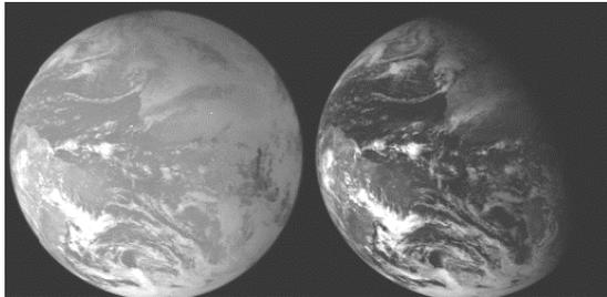
Figure 10. The first image from GERB, left is the total channel and right is the short-wave channel
