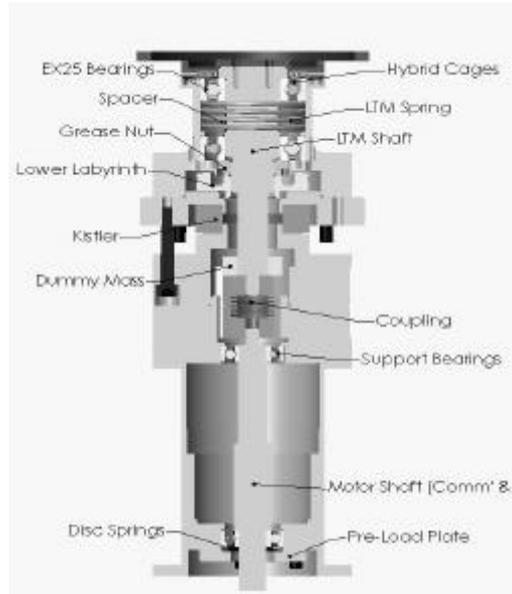
Figure 8: Upgraded LTM Drive Motor and Housing
