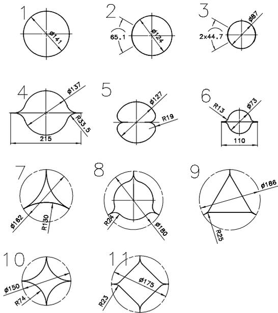
**Fig. 1 possible boom sections**
