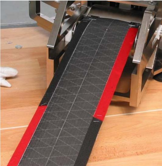
**Fig. 9 CFRP-Segment ready for winding up**
