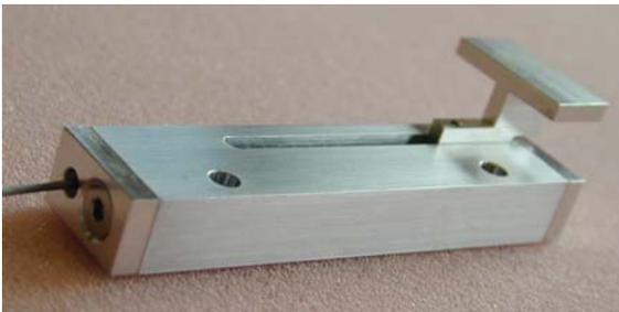
**Figure 5: X and Y actuator pushers**
