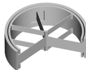
Fig. 5.- Concentric rings with blades in series (CRBS)
