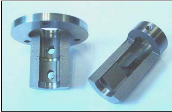
Fig. 21. - Broken pivots after fatigue test.
