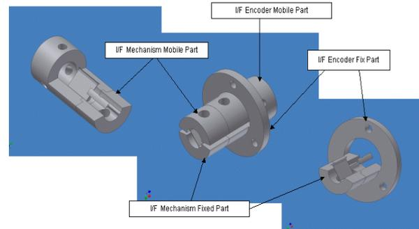
Fig. 8.- Pivot configuration.
