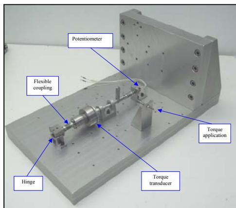
Fig. 12. - Rotational stiffness tooling.
