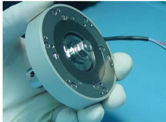
Fig. 10.- Encoder assembled with pivot.
