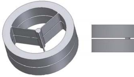
Fig. 6.- Adjacent rings with blades in series (ARBS)
