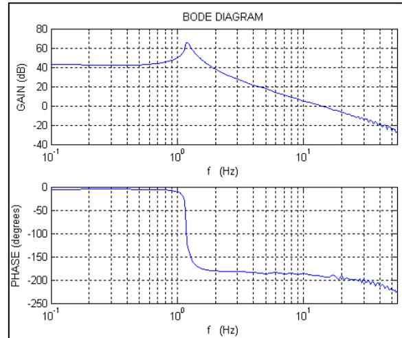
Fig. 16. - Bode diagram open loop of the system : demanded current vs. Angular position (deg/A).
