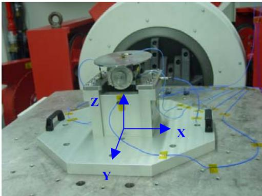
Fig. 18. - Y-axis vibration test.
