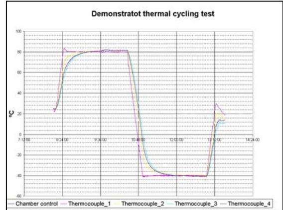
Fig. 19. - Thermal cycle for functional tests.
