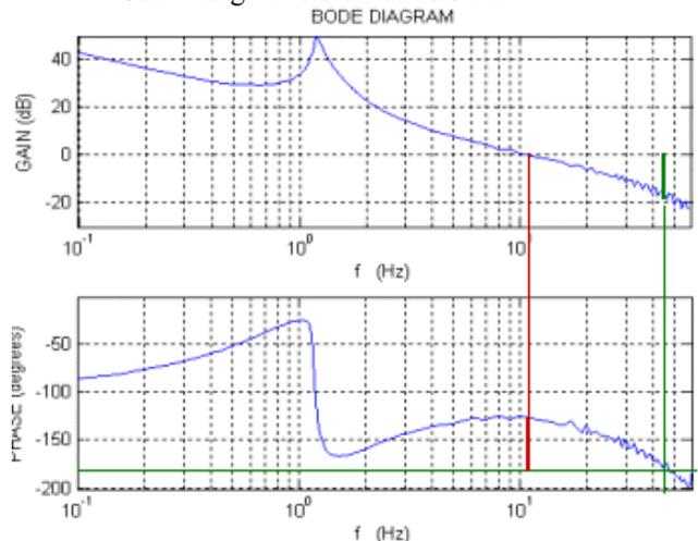
Fig. 17. - Controller and system Bode diagram.
