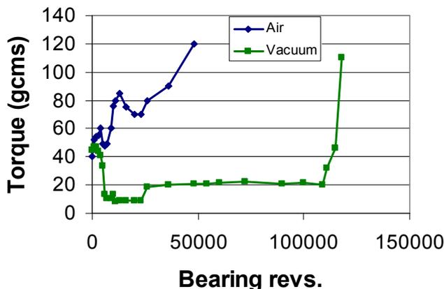
Figure 12: Bearing torque test results in air and in vacuum
