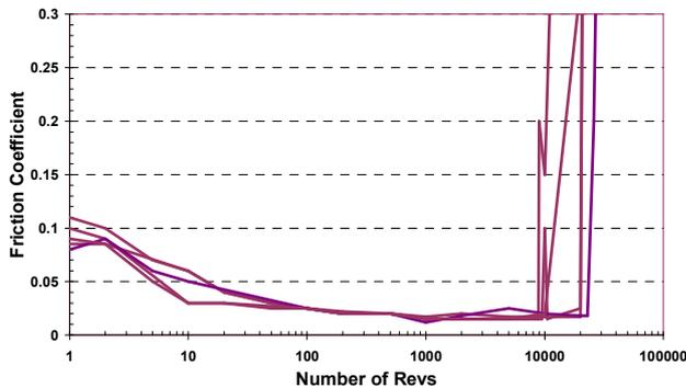
Figure 1: Test results – Supplier A (dry nitrogen)
