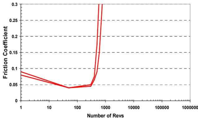
Figure 2: Test results – Supplier B (dry nitrogen)
