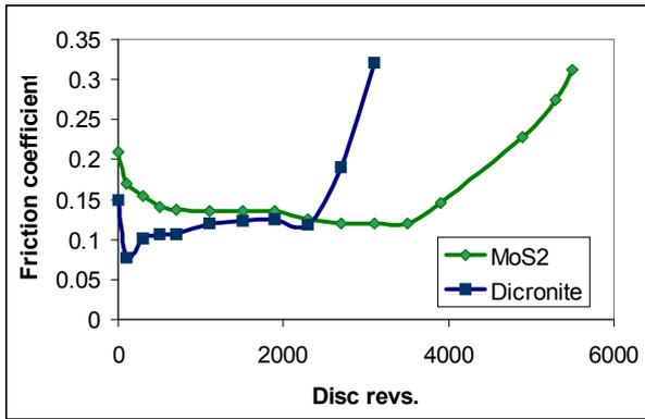
Figure 6: Pin-on disc data for Dicronite in air (corresponding data for sputtered MoS<sub>2</sub> is also shown)
