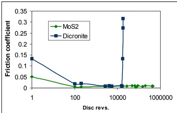
Figure 7: Pin-on disc data for Dicronite in vacuum, compared with sputtered MoS<sub>2</sub>
