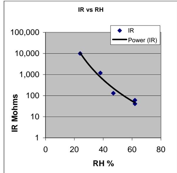
Figure 5: IR vs RH plot, multiple ccts
