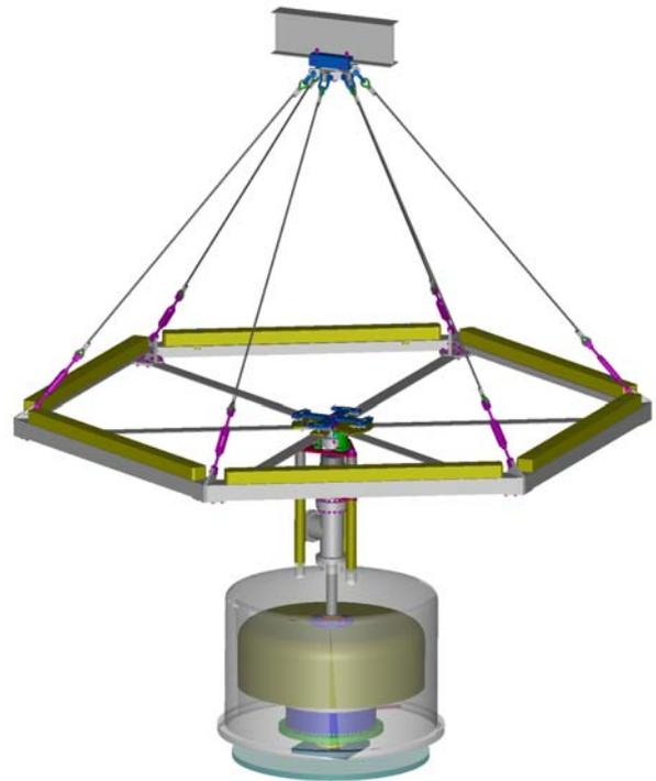
Figure 8: Solar Array Simulator above Thermal Vacuum test chamber
