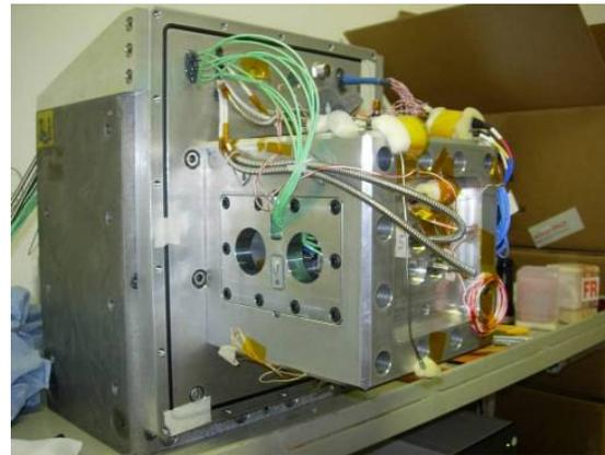
Figure 13. CM caging TM integrated into the vibration fixture. The Vacuum Cover is removed.
