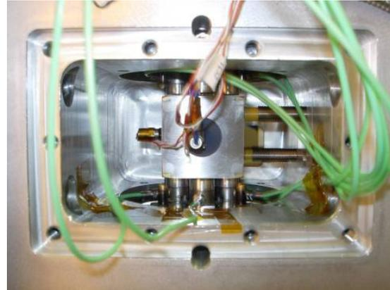
Figure 12. TM and CM integrated into the vibration fixture with sensors for acceleration, position and adhesion force measurements
