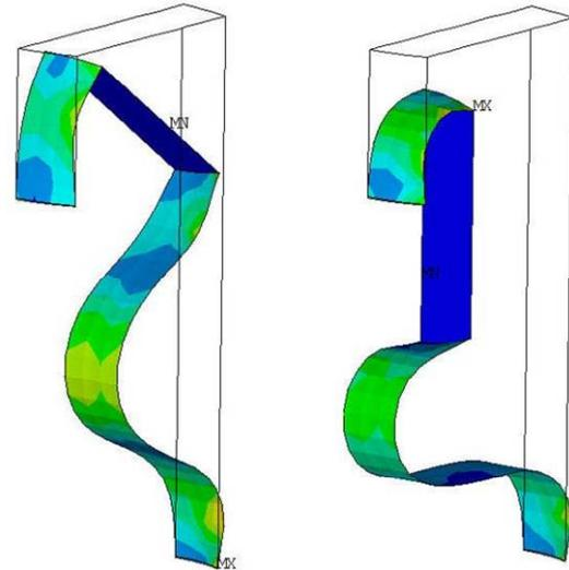
Figure 6. Folding simulation
