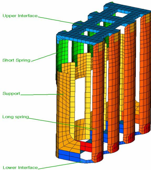
Figure 9. FE-Model for stiffness and thermal simulation
