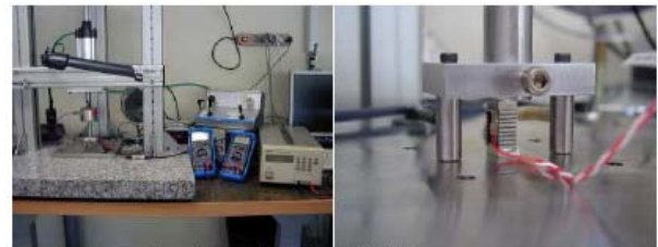
Figure 4. Test bench for blocked force measurement
