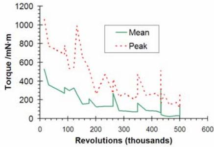
Figure 15 Results from life test of hybrid cage with PGM-HT inserts, without lubricant coating on balls and races.
