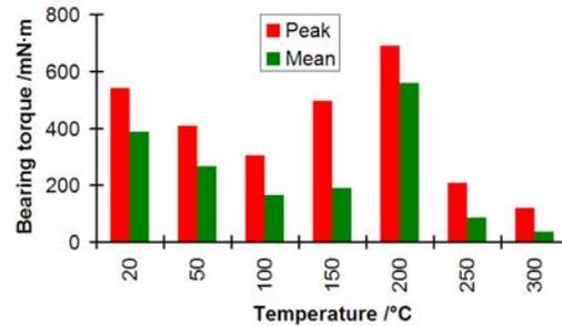
Figure 6 Repeat tests of MoS<sub>2</sub> lubricated bearing with PGM-HT cages with cut - torque measurements at various temperatures.
