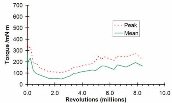
Figure 7 Life test of MoS<sub>2</sub> lubricated bearing with PGM-HT cages with cuts.
