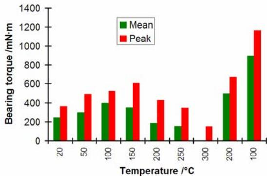
Figure 5 Results of Initial tests of MoS<sub>2</sub> lubricated bearing with PGM-HT cages.
