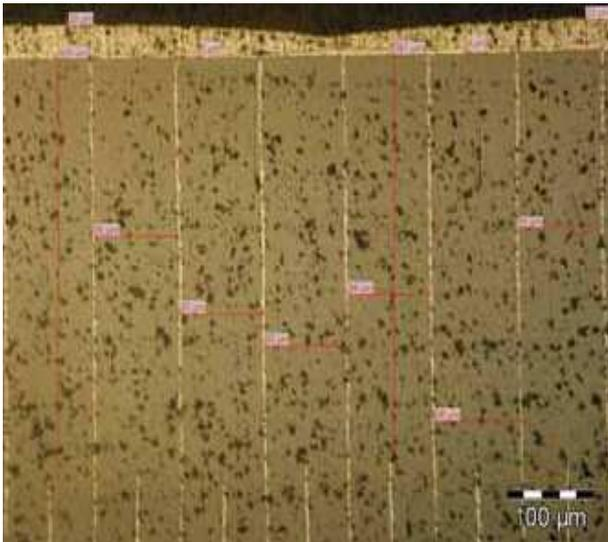
Figure 5: Sectional view of the piezo component
