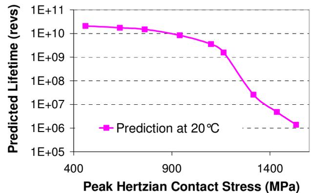
Figure 1. Predicted Bearing Lifetime for Self-Lubricating Bearings v Peak (Ball-Raceway) Hertzian Contact Stress
