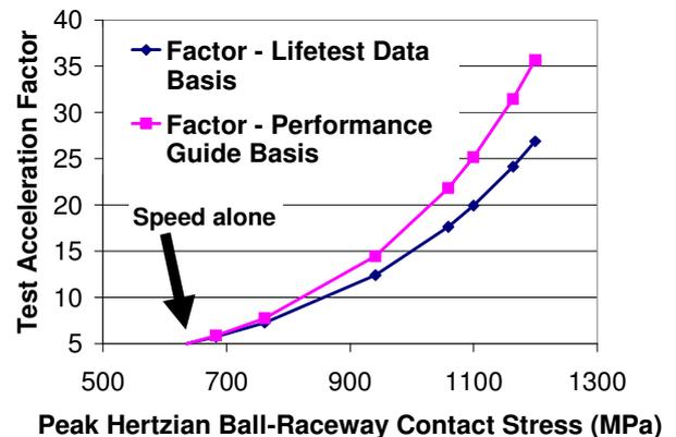
Figure 5 - Test Acceleration Factor Achievable v Ball Raceway Peak Hertzian Contact Stress (assuming "speed alone" acceleration factor of 5)
