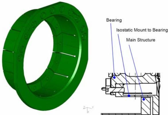
Figure 6. Isostatic Mount to Bearing.
