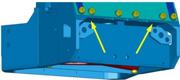
Figure 10. Cut-Out at Kinematic Mount Interface.
