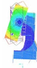
Figure 12. Mode Shape of Wheel Rotation.
