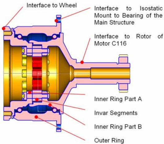
Figure 2. Bearing Cross Section.
