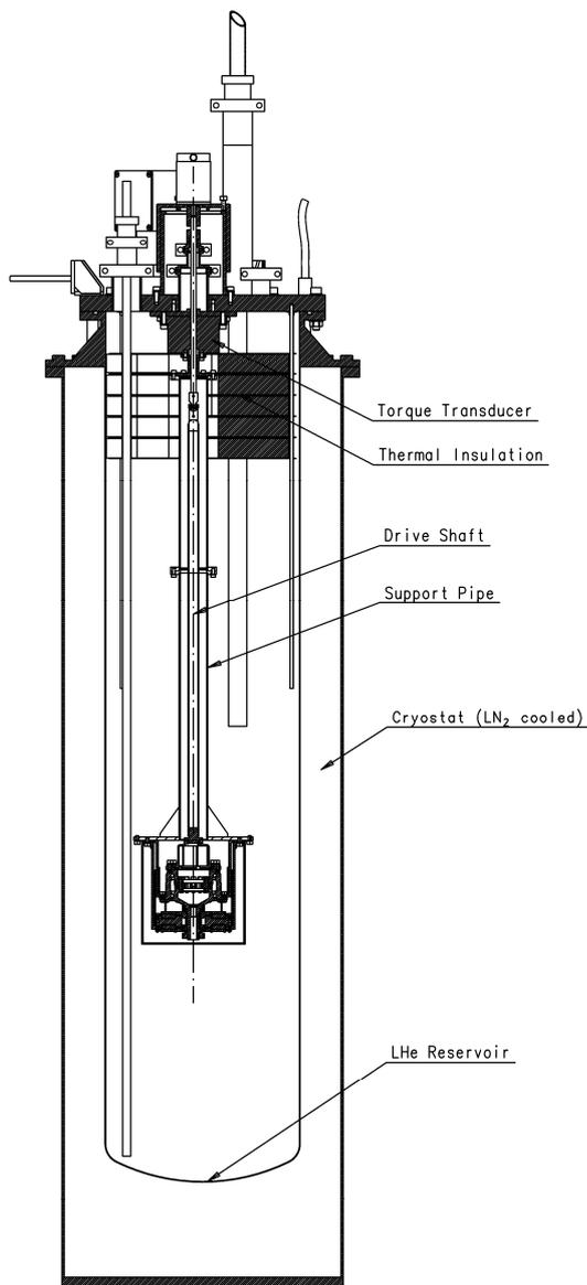
Figure 13. Cryogenic Friction Torque Test Setup.
