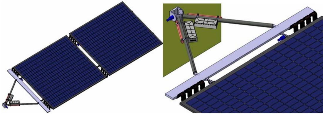
*Figure 4. SA wings with assembled SeCDeS.*
