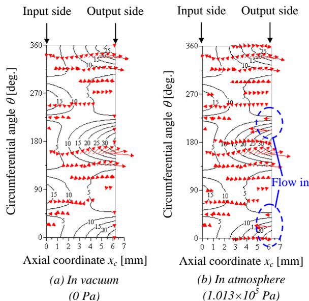
Figure 17. Distribution of oil film thickness and flow vector (unit of contour line:  $\mu\text{m}$ )
