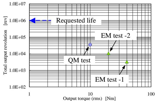
Figure 11. Results of EM and QM life tests
