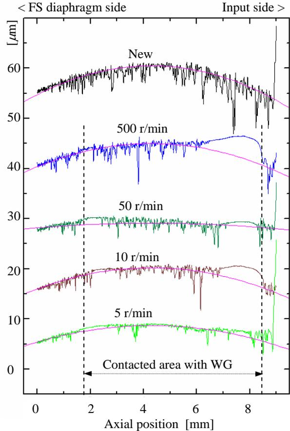
Figure 4. Surface profile of FS inside wall after running test in atmosphere
