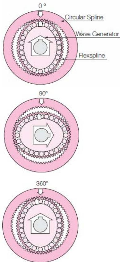
Figure 2. Principle of operation
