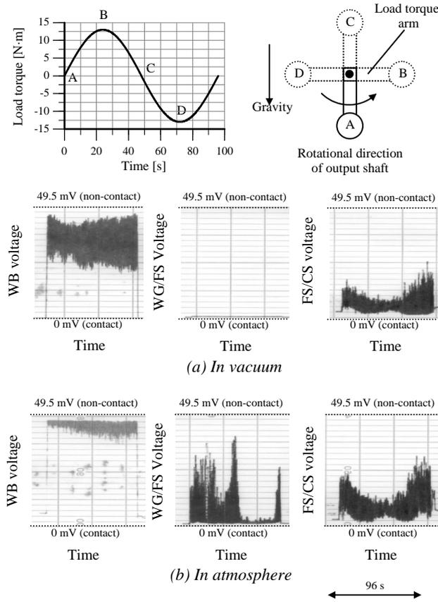
Figure 14. Lubricating conditions at input rotational speed of 100 r/min and load torque of 13 N·m
