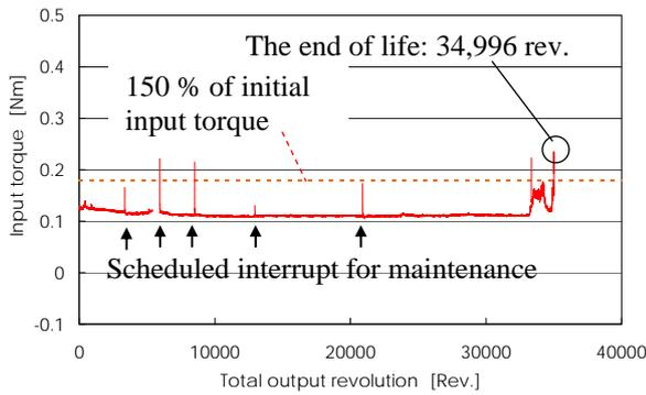
Figure 8. Input torque during life test (at 90 degree of the arm angle)
