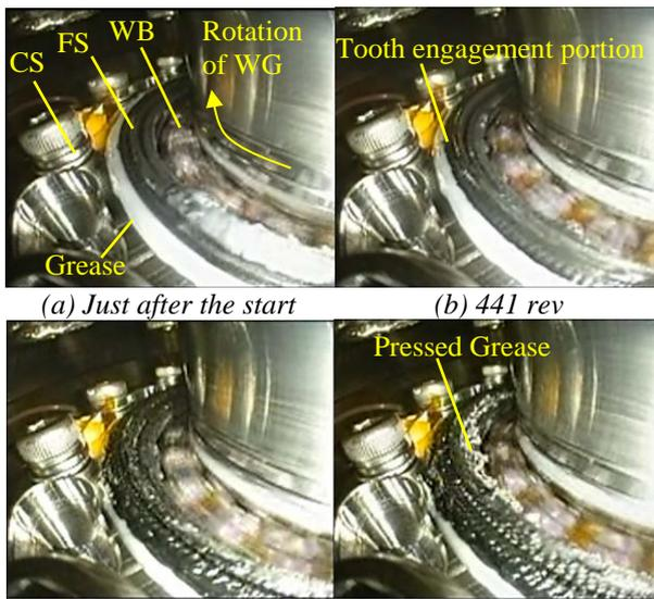
Figure 9. Inside of the test jig observed by fiberscope
