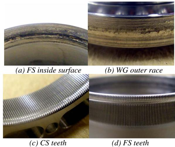
Figure 10. Condition of rubbing surface after life test
