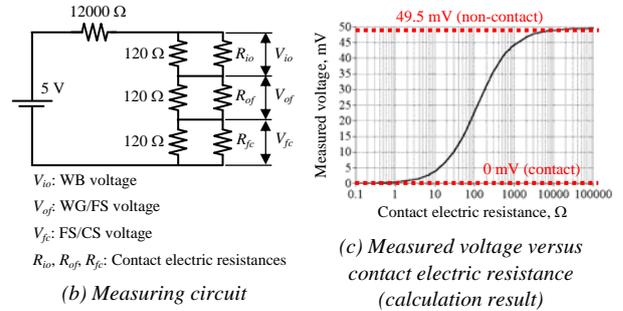
Figure 13. Measuring method of contact electric resistances in SWG
