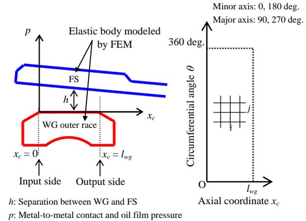
Figure 16. Mixed lubrication analysis model
