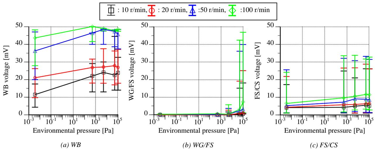
Figure 15. Effects of environmental pressure and input rotational speed on the lubricating conditions at load torque of 13 N·m (0 mV: contact, 49.5 mV: non-contact)
