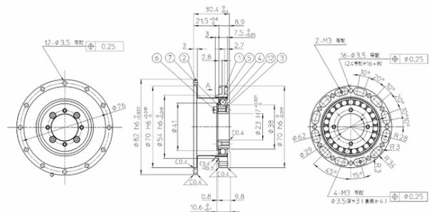
Figure 3. Configuration of the SWG
