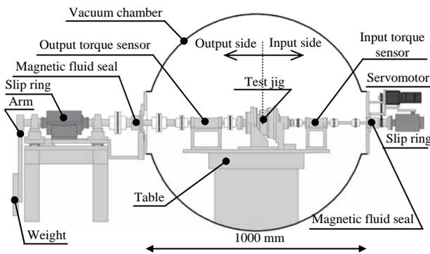
Figure 12. Schematic of experimental apparatus
