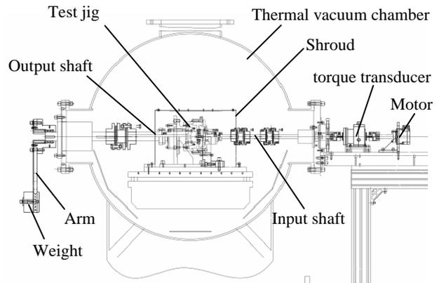
Figure 7. Thermal vacuum test equipment
