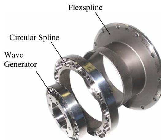
Figure 1. SHF type strain wave gearing
