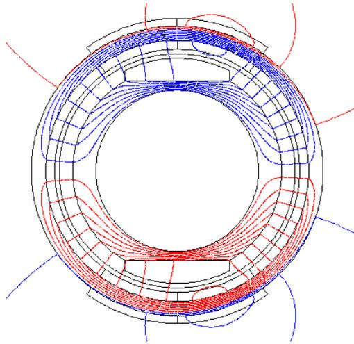
Figure 1: View of the Flux line created by the coils
