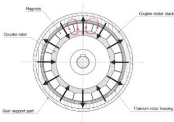
Figure 3. Cross-section of gear motor at coupler
