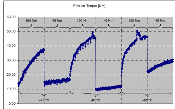
Figure 6. Dry gear friction torque during life testing
