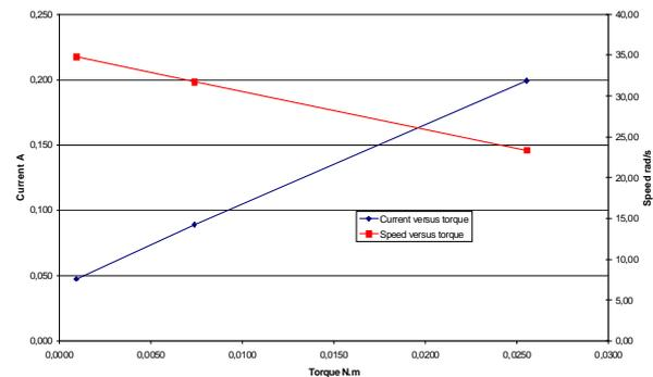
Figure 7. Measured motor characteristic
