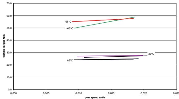
Figure 9. SBGM friction torques
