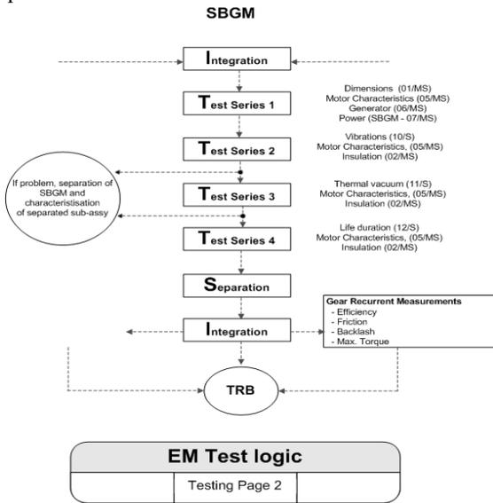
Figure 8. Gear motor test sequence
