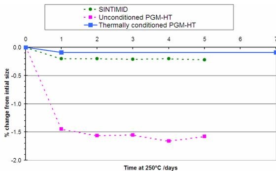
Figure 3. Dimensional change of dummy PGM-HT cages after heating to 250 °C – showing beneficial effects of pre-conditioning on PGM-HT. [4]
