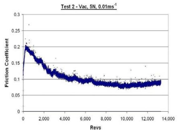
Figure 6. Test 2 – Vacuum, 5N,  $0.01\text{ms}^{-1}$
