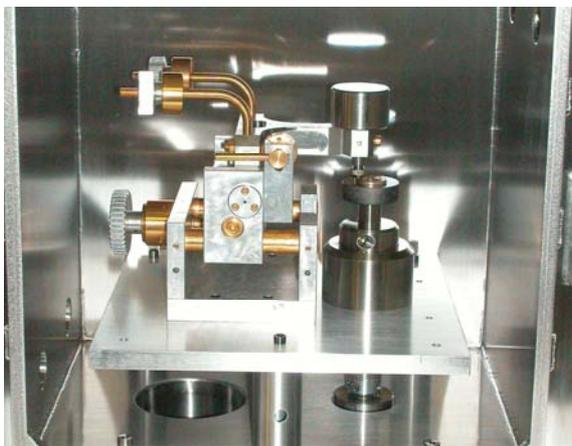
Figure 4. Vacuum pin on disc tribometer
