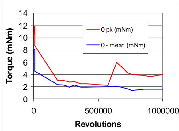
Figure 12. Test 24 results, with MoS<sub>2</sub>-coated bearings
