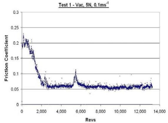
Figure 5. Test 1 – Vacuum, 5N,  $0.1\text{ms}^{-1}$
