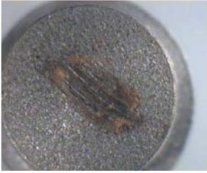
Figure 8. Wear scar after air test
