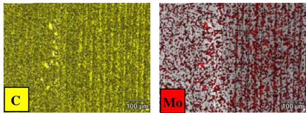
Figure 7. EDX maps of the disc surface of the after test against MoS<sub>2</sub> filled PEEK at -80°C
