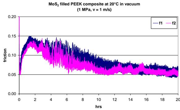
Figure 4. Friction vs. time of MoS<sub>2</sub> filled PEEK composite in vacuum at 20°C
