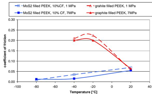
Figure 2. Coefficient of friction of MoS<sub>2</sub> filled PEEK in vacuum environment ( $v = 0.1 \text{ m/s}$ )
