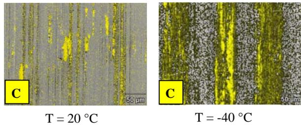
Figure 8. EDX maps of the disc surface of the after test against graphite filled PEEK
