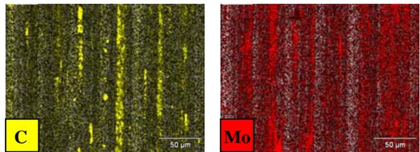
Figure 6. EDX maps of the disc surface of the after test against MoS<sub>2</sub> filled PEEK at 20°C
