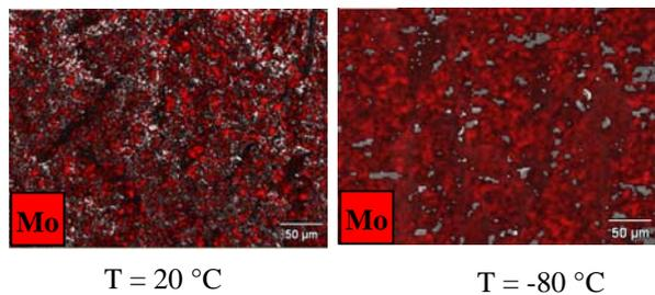
Figure 7. EDX analyses of MoS<sub>2</sub> filled PEEK composite pin at 1 MPa
