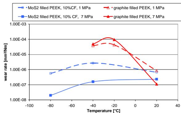
Figure 3. Wear rate of MoS<sub>2</sub> filled PEEK in vacuum environment ( $v = 0.1 \text{ m/s}$ )
