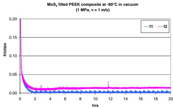
Figure 5 Friction vs. time of MoS<sub>2</sub> filled PEEK composite in vacuum at -80°C
