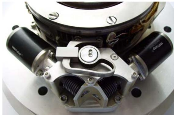
Figure 5. Breadboard Model of Differential Worm Drive
