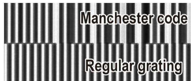
Figure 3. Image of a double-track linear scale consisting of a 12 bit Manchester code and 100um regular grating. Image obtained by ultra-compact USB camera and shadow imaging.
