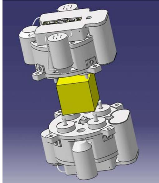
Figure 2: Caging mechanism
