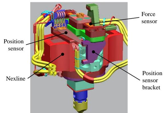
Figure 7: Location of force and position sensor
