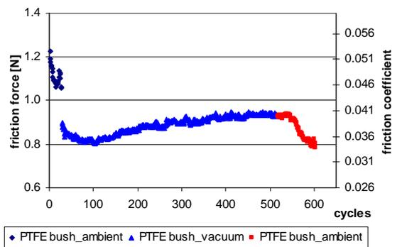
Figure 21: Friction coefficient of PTFE coated bushings
