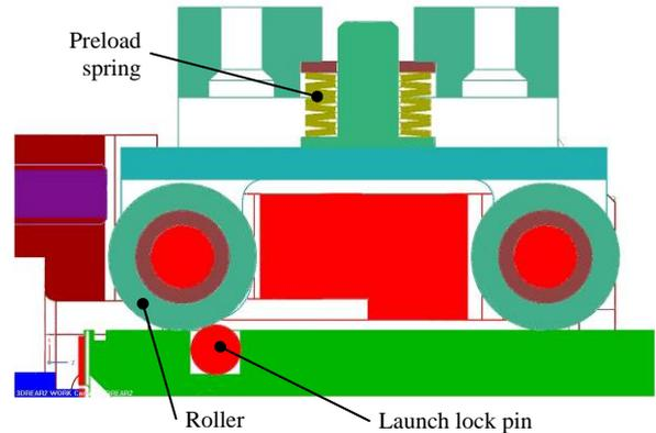
Figure 10: Launch lock consisting of pin and roller
