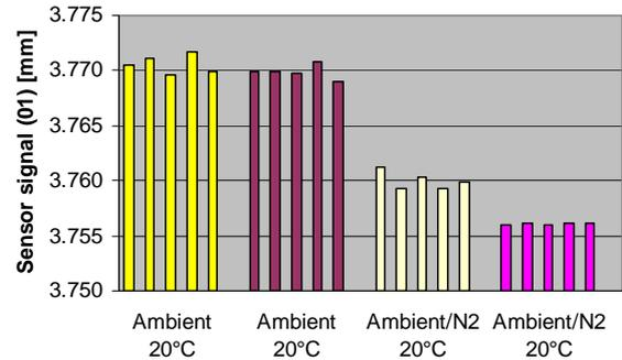
Figure 17: Position sensor signal in different environments
