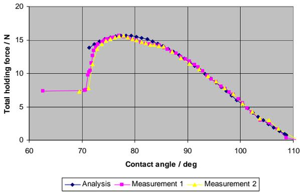
Figure 11: Holding force profile of launch lock
