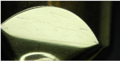
Figure 23: Defects of gold coating
