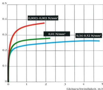
Figure 19: Influence of speed on PTFE friction
