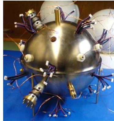
*Figure 10: Stator and rotor integration*
