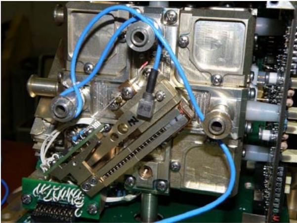
Figure 13 Accelerometer on the Lever of z-axis LM
