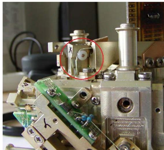
Figure 12 Fiber was broken during some test
