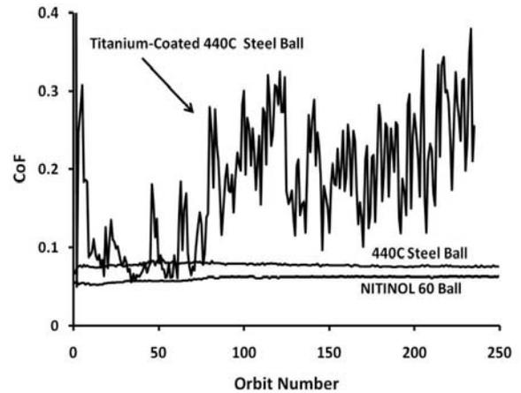
Figure 2. Friction traces for a 440C steel ball, a 440C ball coated with a thin film of titanium and a NITINOL 60 ball, all lubricated with Pennzane 2001A and running on 440C steel plates.
