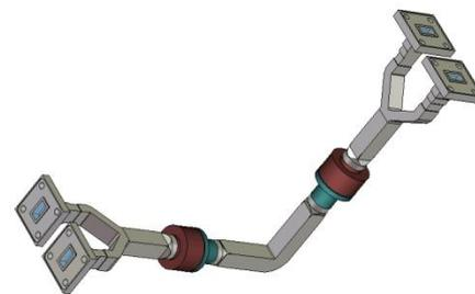
Figure 4: RF-design of the Ka-band rotary joint (developed by NTP)
