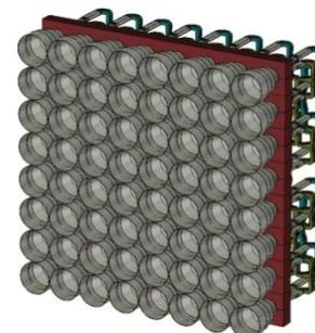
Figure 1: LISA Ka-band antenna with structural plate
