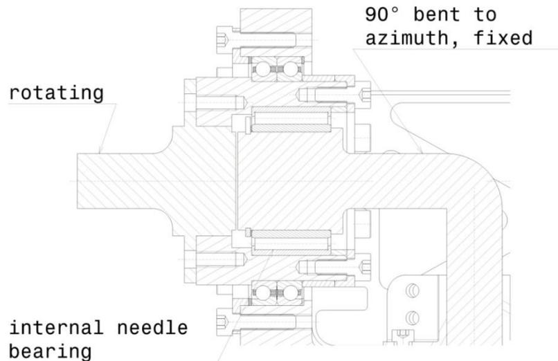
Figure 5: Detail of the elevation RF-rotary joint (simplified)
