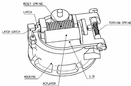
Figure 4: V12 - Linear Latch with Direct Actuation
