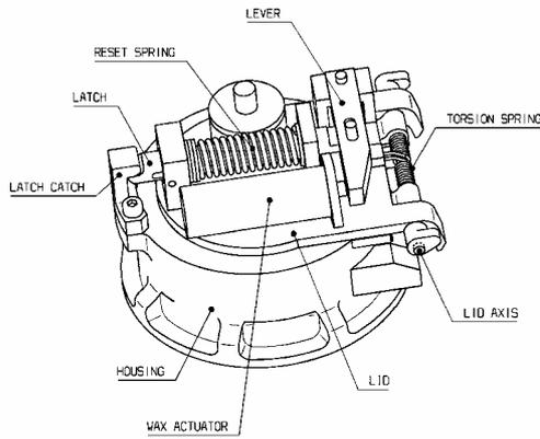
Figure 3: V11 - Linear Latch plus Lever System
