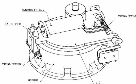
Figure 5: V15 - Rotary Latch
