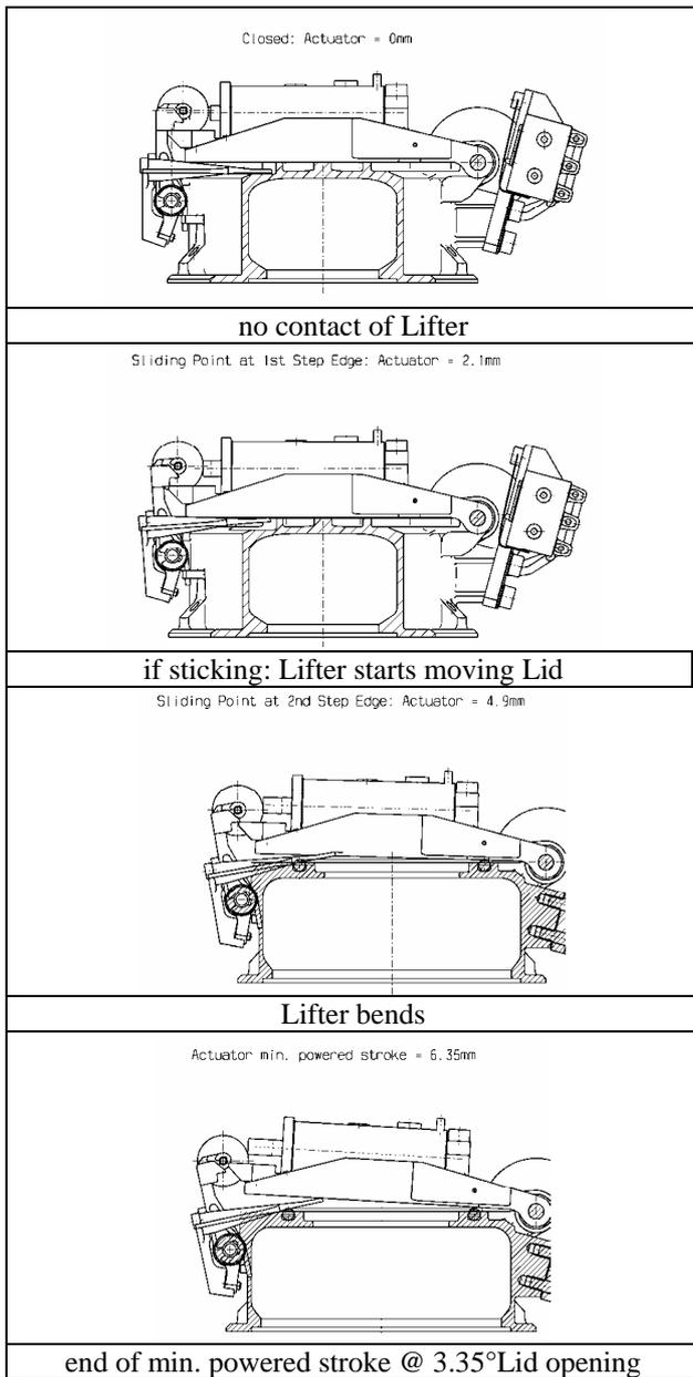
Figure 11: Opening sequence with Lifter
