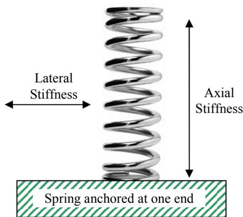
Figure 1.1-1, Spring Characteristics
