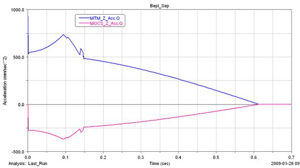
**Figure 1.2-3, The effect of Excess Connector Energy Effect on Module Accelerations**
