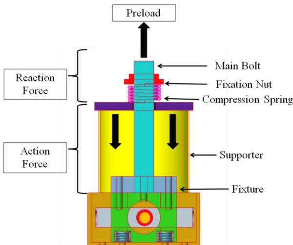
Figure.3 Design and concept of preload generator
