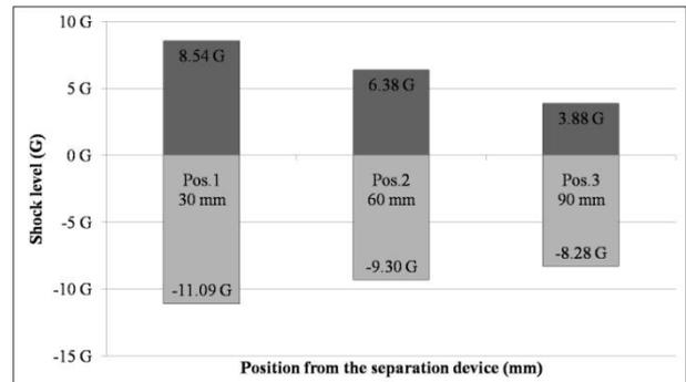
Figure.6 Shock level test result
