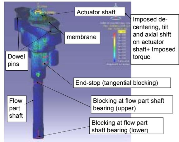
Figure 5. Actuator/flow part coupling
