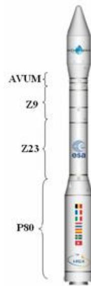
P80, Z23, Z9 and AVUM. (*figure 2*) The TVCs are optimised while keeping the same architecture. Each TVC system consists of two Electro-Mechanical Actuators (EMA), one piloting electronics, called the Integrated Power Distribution Unit (IPDU), the electrical power generation via a Battery Set (BS) consisting of Li-ion battery module(s) and the relevant cable harness for power distribution and telemetry between the Battery, IPDU, EMA and Telemetry (TLM).
