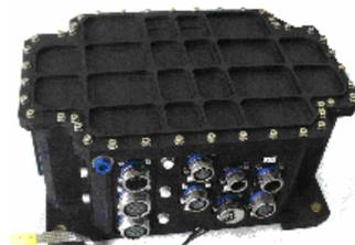
figure 7. A photograph of the fourth stage electronics: AVUM IPDU
