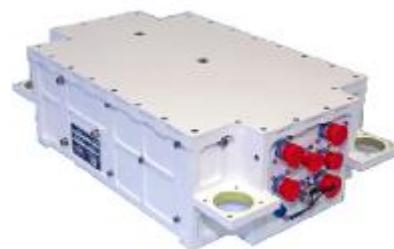
figure 6. A photograph of the second and third stages electronics: Z23 / Z9 IPDU
