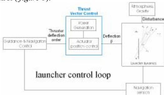
*figure 1. The TVC in the launcher attitude control*
