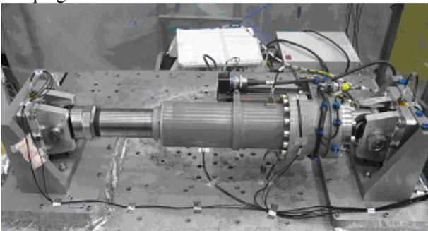
*figure 14. A photograph of the P80 EMA installed on the shaker during qualification vibration.*
