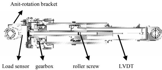
figure 9. cross section of P80 EMA
