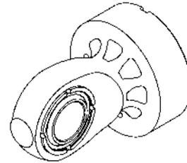
figure 11. Tailstock lug with integrated force sensor
