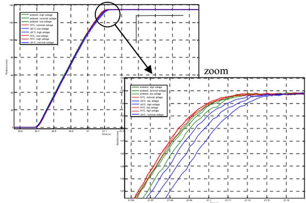
figure 17. P80 EMA maximum step response at different temperatures with different input voltages.
