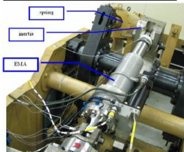
*figure 15. P80 EMA installed in its load test bench*
