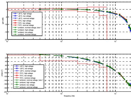
figure 16. P80 EMA frequency response at different temperatures with different input voltages.
