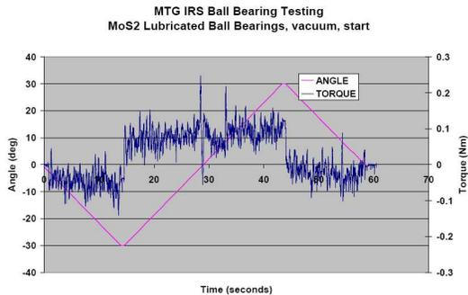
Figure 3: Baseline regeneration profile for MoS<sub>2</sub> lubricated ball bearings in vacuum at the start of vacuum test phase (255 cycles)
