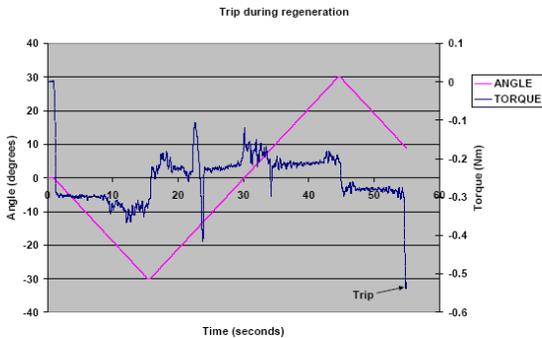
Figure 9: Trip during regeneration at 136,066 cycles (oil-lubricated ball bearings). Transient at approx -15 deg attributable to presence of hard particle in the bearing.
