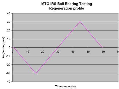
Figure 2: Regeneration profile used in life test programme
