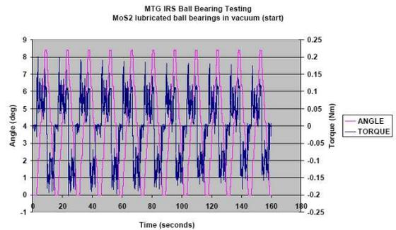
Figure 7: Baseline life test profile for MoS<sub>2</sub> lubricated ball bearings in vacuum
