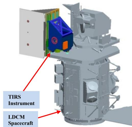
Figure 1. The TIRS instrument on the LDCM satellite
