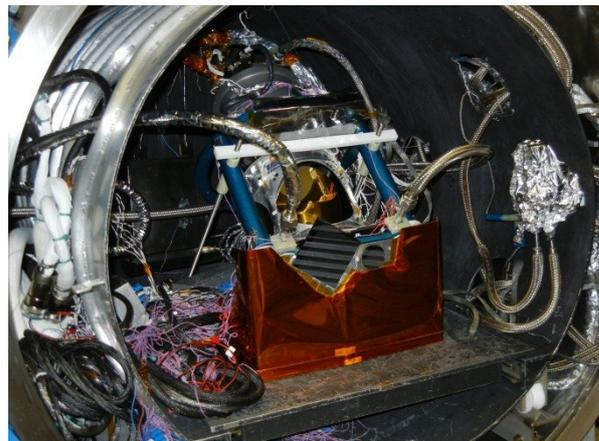
*Figure 4. The SSM in the thermal vacuum chamber, tilted to allow direct horizontal measurement of the scene mirror position against in-chamber reference flats. The gold Scene Mirror is visible between the blue support frame posts.*
