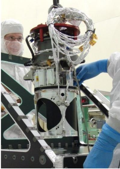
Figure 5. The SSM is lowered into the TIRS instrument
