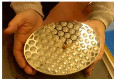
*Figure 3. The back of the Scene Mirror before polishing*
